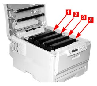
**3.** Pull the colored toner release lever on the cartridge to be replaced towards the front of the printer. Shown: replacement of the black toner cartridge
